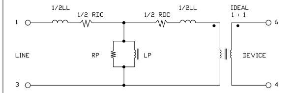
RDC : SUM OF WINDING RESISTANCES, CAUTION : DO NOT PASS DC ON COMPLETED TRANSFORMERS.
