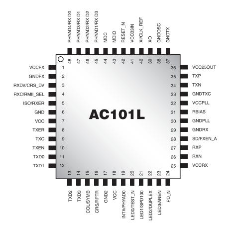
The **AC101L** provides all of the required features of an MII compliant 10/100TX/FX Ethernet transceiver. The **AC101L** has the lowest power consumption of any other single- port solution.
