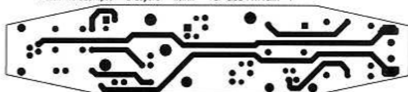
Atech-A1f028A.pcb - 2 Layers - 1.6mm TOP SIDE PATTERN -1
